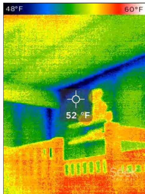
11.1 Item 4(Picture) Chilled corners at exterior walls
